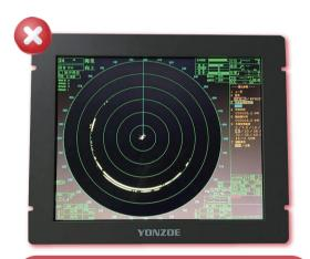
Incorrect setting:Unable to show the radar performance falls 10dB
